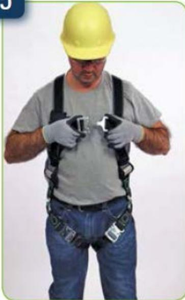
Connect chest strap and position in midchest area. Tighten to keep shoulder straps taut.
