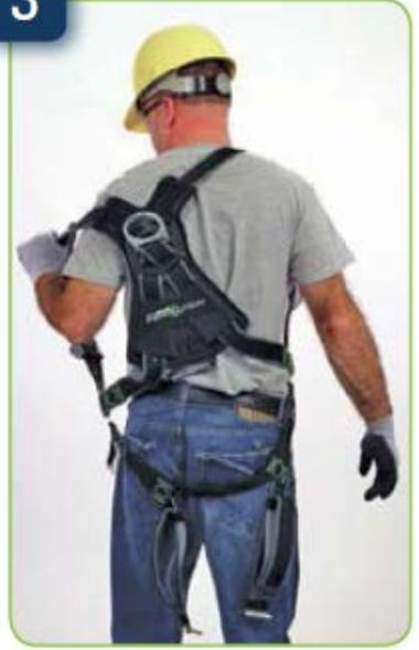
Slip straps over shoulders so D-ring is located in middle of back between shoulder blades.
