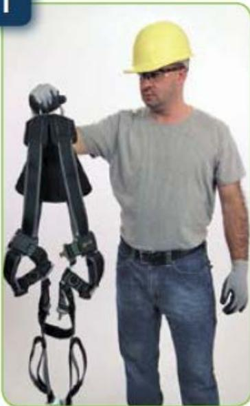
Hold harness by back D-ring. Shake harness to allow all straps to fall in place.
