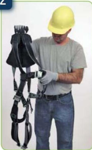
If chest, leg and/or waist straps are buckled, release straps and unbuckle at this time.
